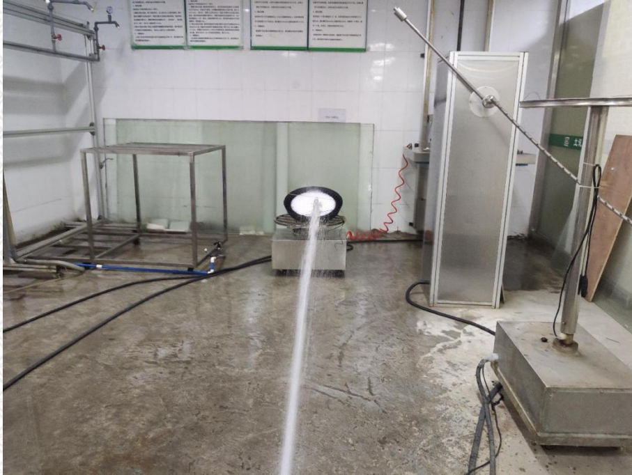
Photo 19: IPX6 test of model GL-UFO500-J
