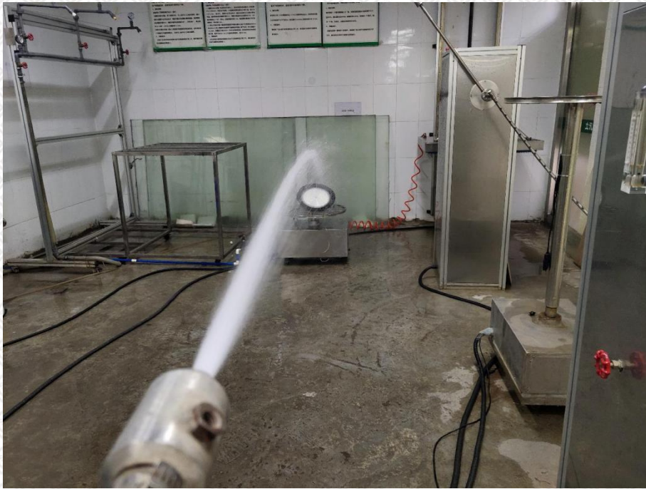
Photo 9: IPX6 test of model GL-UFO200-C
