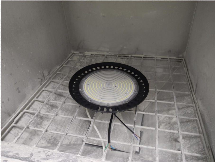
Photo 13: IP6X test of model GL-UFO200-K
