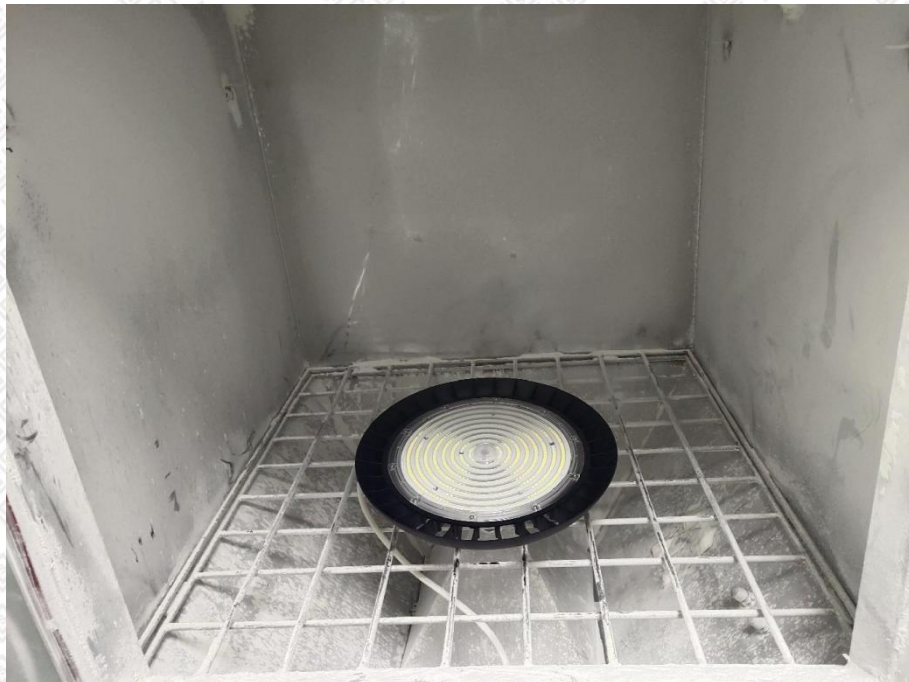
Photo 8: IP6X test of model GL-UFO200-C
