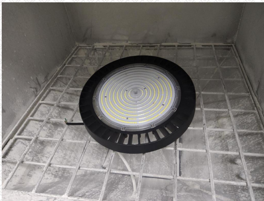
Photo 3: IP6X test of model GL-UFO240-N
