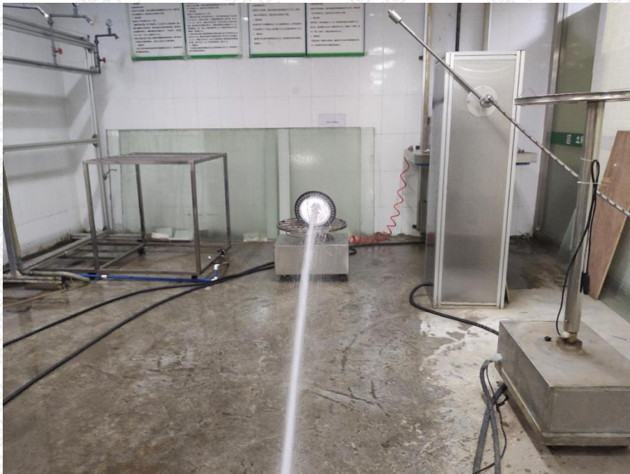
Photo 14: IPX6 test of model GL-UFO200-K
