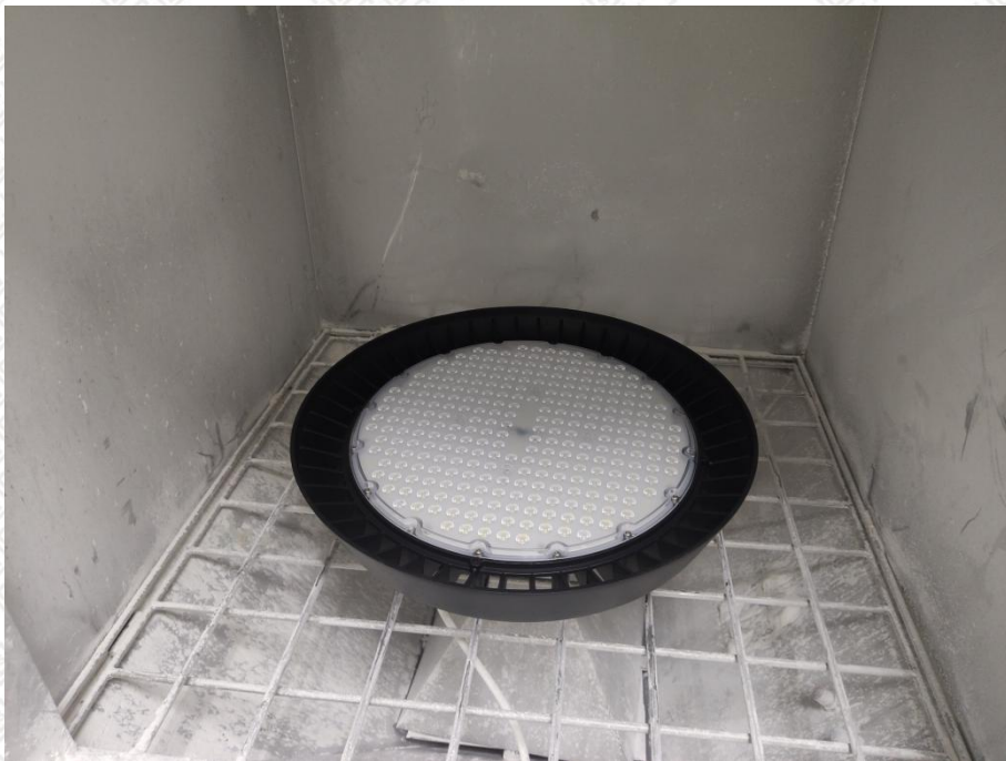
Photo 18: IP6X test of model GL-UFO500-J
